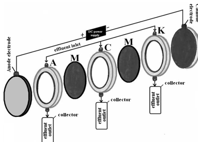
Fig. 1. Scheme of mini-laboratory electro dialysis cell with three compartments and membrane A - anodic compartment, C - central compartment, K - cathodic compartment, M - membrane
